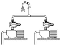
Two PRESSCONTROL devices with different restart pressure calibrations (T 1.2 bar and T 1.5 bar)
