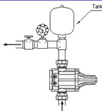
For minimal delivery demands, the application of a small expansion tank downstream from the PRESSCONTROL allows for reducing the pump start-ups.
