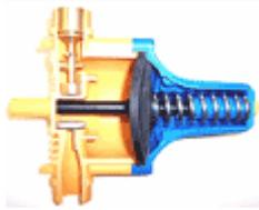
Body, non-return valve, rear part and safety valve are moulded in 30% fibreglass reinforced polyamide 6 (PA6GF30).
